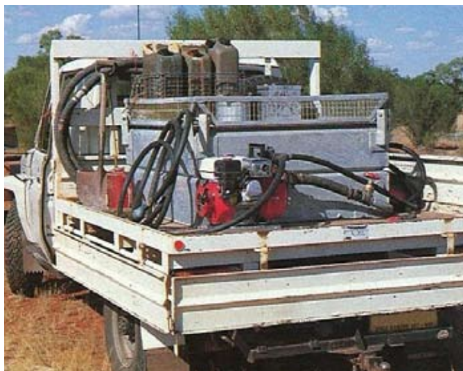
A well equipped fire unit with a tank and reliable pump unit, hoses with adjustable nozzles, drip torches and UHF radio. Photo: K.K. Holmes.
